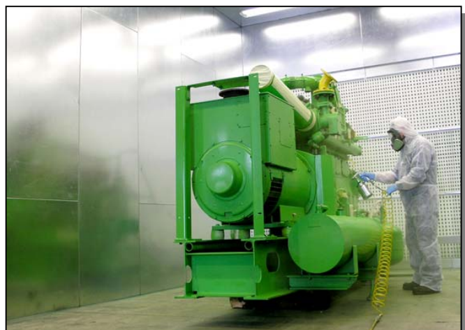
Jenbacher J208 engine under re-spray after major overhaul
